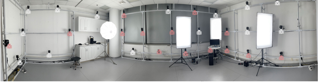
Figure 8. Dome setting, the red cameras are zoomed cameras for capturing hands, and other white cameras are wide-angle cameras for capturing the full body.
