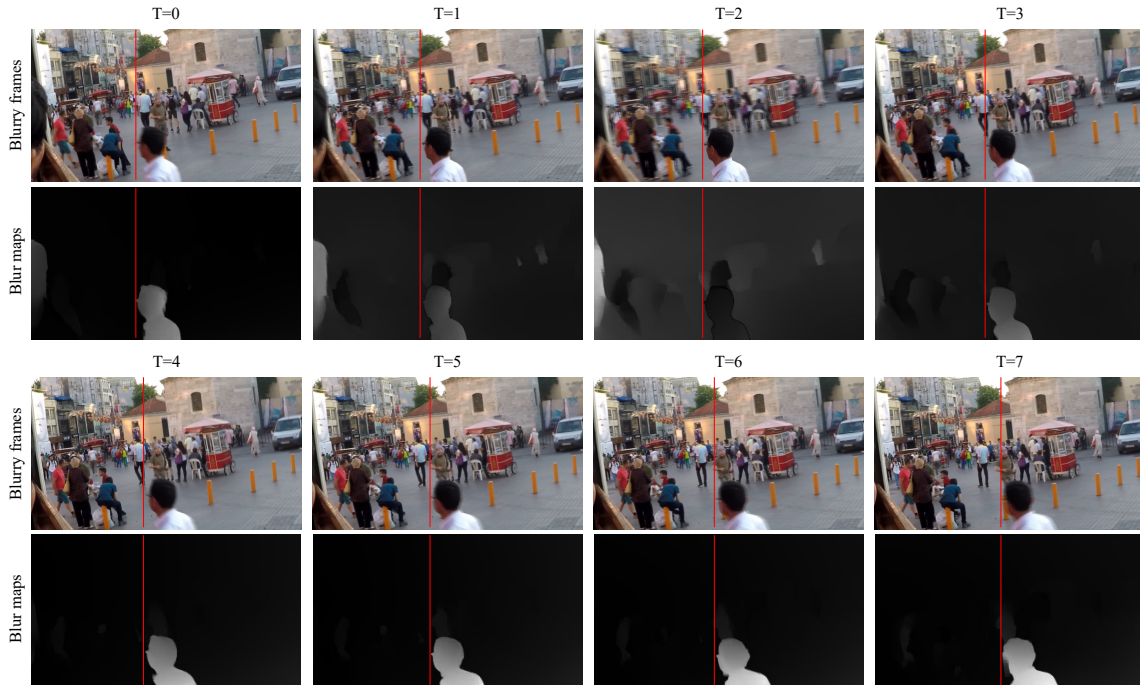
Figure 2. Visual results of blur maps and corresponding blurry frames on GoPro dataset. Specifically, we provide the visual results for a sequence length of 8 frames. In the blur maps, a higher weight indicates that the corresponding region in blurry frame is more blurred. The visual results demonstrate that our blur maps accurately provide the information about blurry regions in blurry frames.
