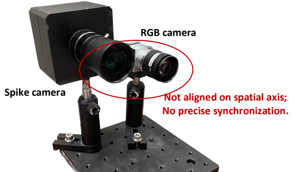
Figure 4. Illustration of the built simple spike-RGB camera system for capturing real-world scenes.
