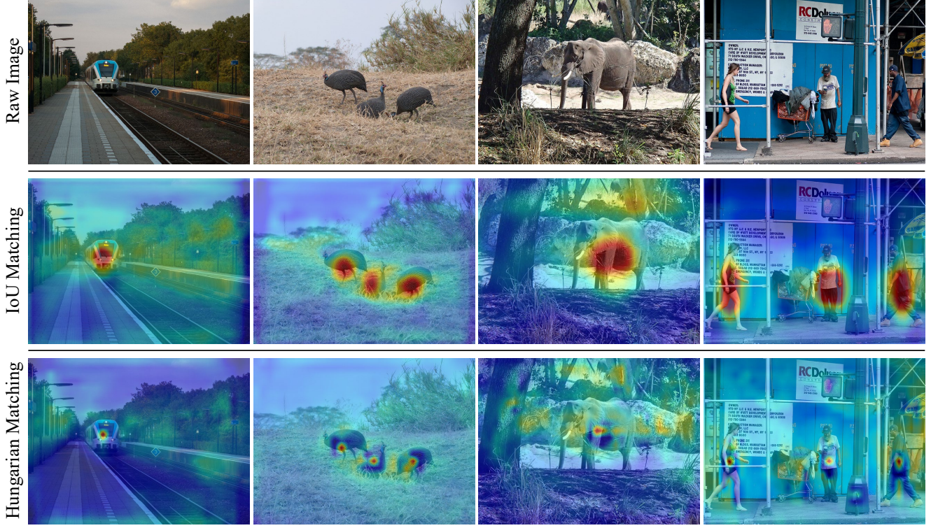
Figure 4. Visualizations of the activation maps generated by variants of Faster R-CNN using either IoU matching (the second row) or Hungarian matching (the third row).
