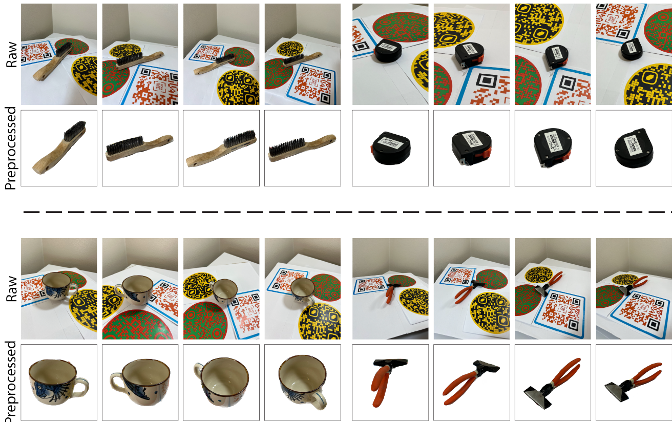
Figure 2. Visualization of raw and preprocessed multi-view images. Raw images represent the images directly output from the capture device, i.e., iPhone 13 Pro. We process raw images with segmentation and cropping before feeding them into the models. For more implementation details, please check Section 5 in the main paper.
