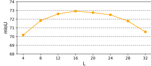
Figure 1. mIoUs when setting L to different values. We choose L=16 as our final setting.
