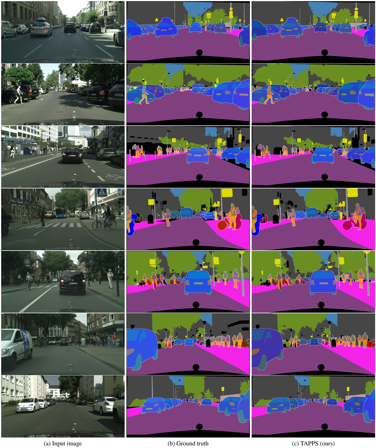
Figure 8. TAPPS with Swin-B [11] on Cityscapes-PP [3, 4]. The Swin-B backbone is pre-trained on COCO panoptic [10]. White borders separate different object-level instances; color shades indicate different categories. Note that the colors of part-level categories are not identical across instances; there are different shades of the same color. Best viewed digitally.
