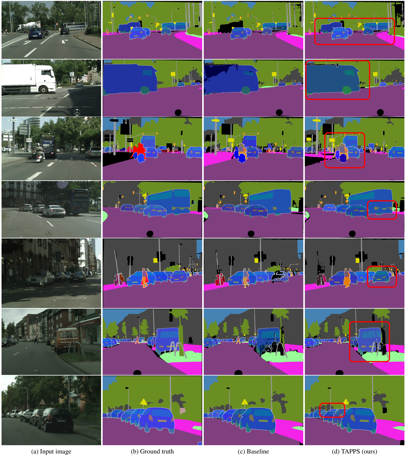
Figure 4. Qualitative examples of TAPPS and our strong baseline on Cityscapes-PP [3, 4]. Both networks use ResNet-50 [6] with COCO pre-training [10]. White borders separate different object-level instances; color shades indicate different categories. Note that the colors of part-level categories are not identical across instances; there are different shades of the same color. In these examples, we can see how TAPPS improves both the instance separability and part segmentation quality with respect to the strong baseline. The red boxes indicate regions in which these differences are best visible. Best viewed digitally.
