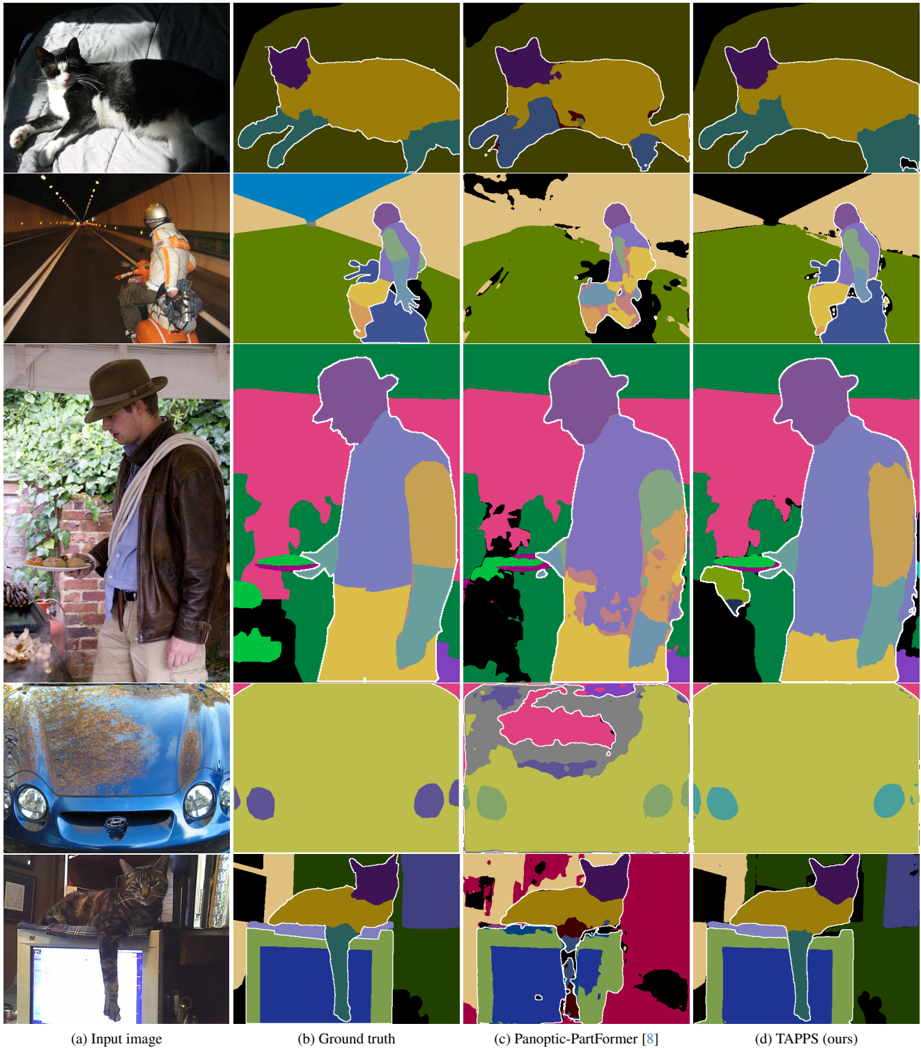
Figure 5. Qualitative examples of TAPPS and Panoptic-PartFormer [8] on Pascal-PP [1, 4, 5, 14]. Both networks use ResNet-50 [6] with COCO pre-training [10]. White borders separate different object-level instances; color shades indicate different categories. Note that the colors of part-level categories are not identical across instances; there are different shades of the same color. Best viewed digitally.
