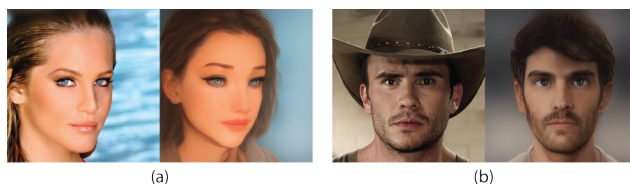
Figure 11. Failure examples. (a) inconsistent gaze directions, (b) unmodeled hat.
