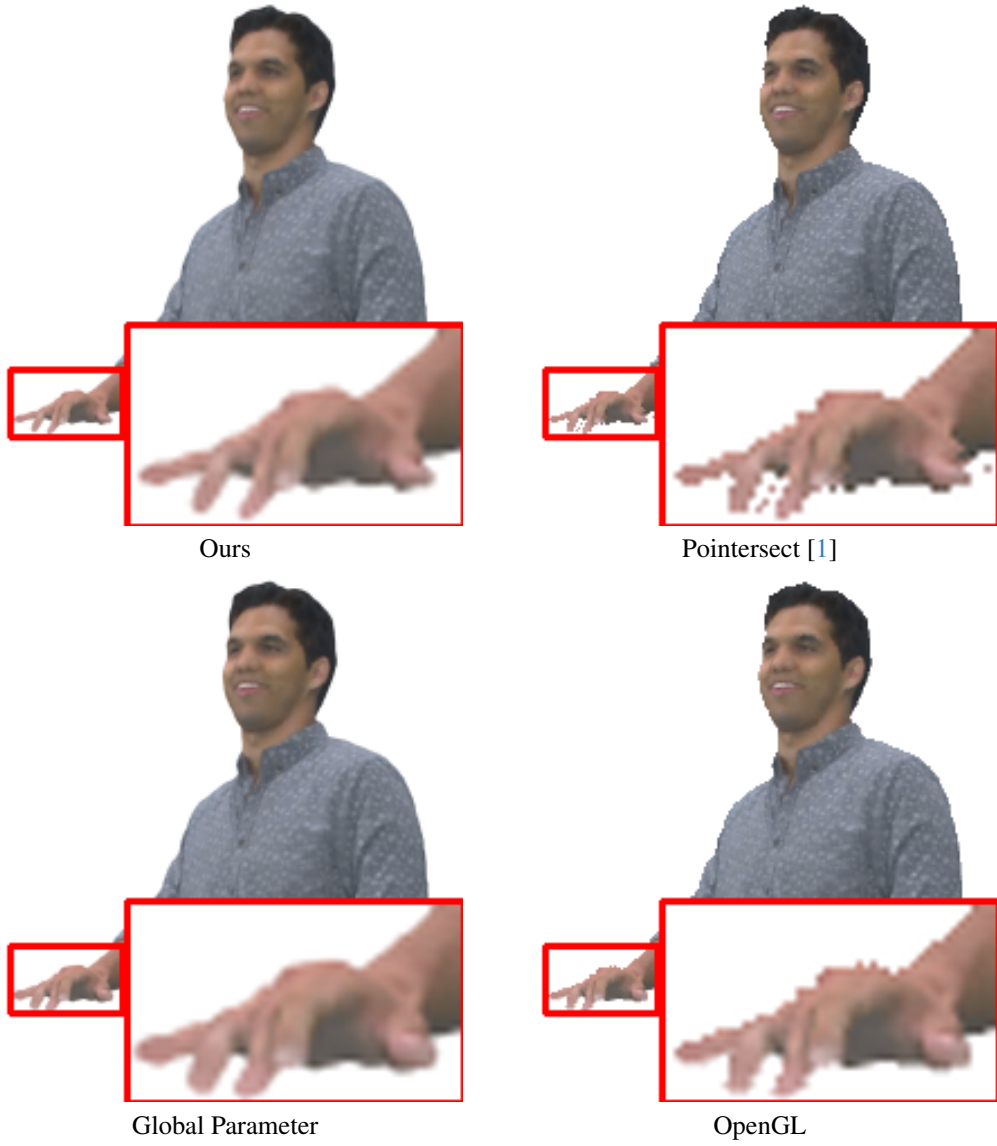
Figure 2. Rendering results of different methods on the sequence Loot (610 K points, 23 Mbps) in the 8iVFB database. The insets visualize local details with 3\times zooming.
