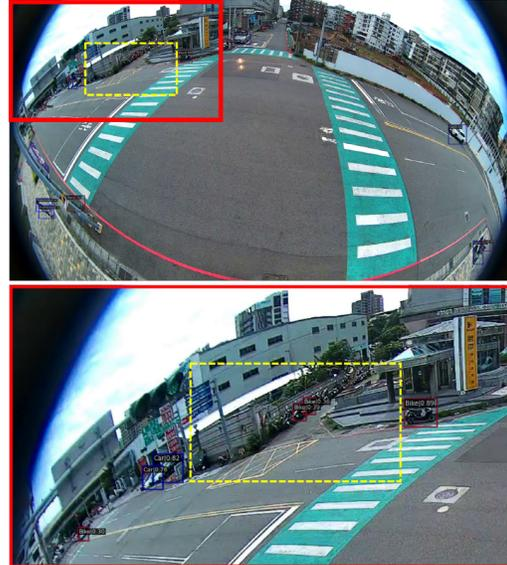
Figure 3. An example of sliced inference. The region corresponding to the red box in the above image is resized to match the model’s input size (as shown in the bottom image) before being inputted. As a result, the small objects within the yellow box are greatly enlarged, allowing the model to detect the target objects more accurately.
