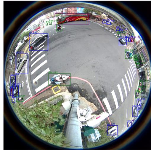
Figure 1. An example of road object detection using fish-eye cameras. The objective of this task is to detect bus, bike, car, pedestrian, and truck objects from images captured by fish-eye cameras.
