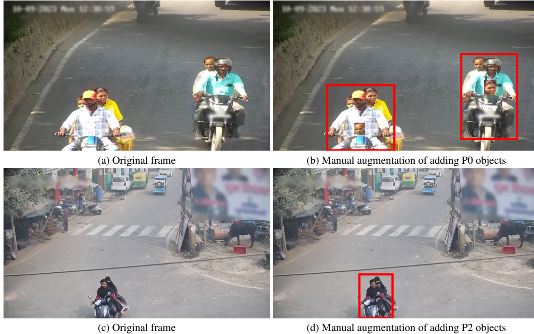
Figure 2. Illustration for our manual augmentation method, where figures 2a and 2c show original frames, while figures 2b and 2d demonstrate samples generated by our manual augmentation of adding P0 and P2 objects.
