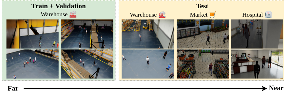
Figure 3. Samples from the AIC24 Multi-Camera People Tracking dataset . This illustration showcases sequences across training, validation, and test sets, including warehouse, market, and hospital environments. The dataset is composed of synchronized videos from 8 to 16 distinct camera angles, each spanning over 13 minutes, highlighting challenges such as non-overlapping regions , varying occlusion conditions , and the need for cross-domain generalization in multi-camera tracking systems.
