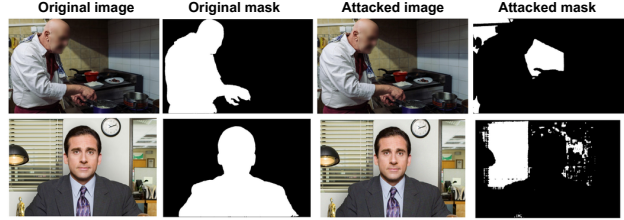
Figure 5. Examples of attacks with perturbations small enough to be imperceptible by the human eye, created using an FGSM-based approach. The attack successfully destroys the original masks.
