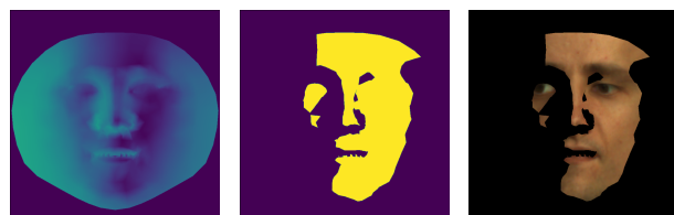
Figure 5. Example of a computed UV angle frame \Theta_{UV} , the subsequent UV appearance mask for \Theta_{UV} < 45^\circ and resultant masked UV appearance frame to be provided to the video-based model from PURE [33].
