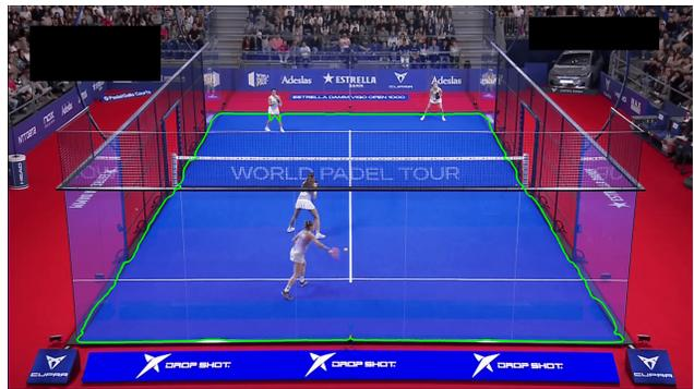
Figure 3. Color-based field extraction for approximating corner positions. Interference from the environment causes inaccurate corner approximations along the contour of the court (green line).
