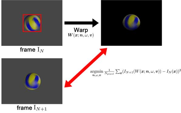
Figure 8. Overview of the image-based baseline method. It warps the pixels on the ball and optimizes to minimize the MSE between the warped pixels and pixels on the adjacent frame.
