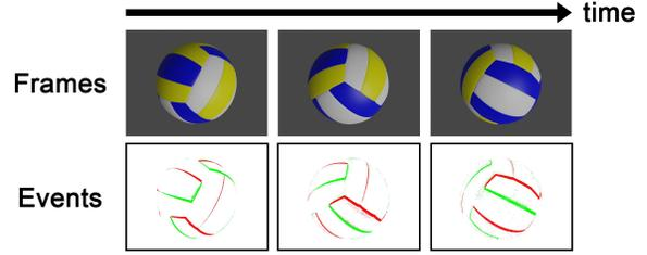
Figure 3. Events that occur when the ball spins. Events are concentrated around the edges on the image.
