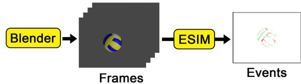
Figure 7. Dataset synthesis. The frame rendered in Blender is input to ESIM to generate events.
