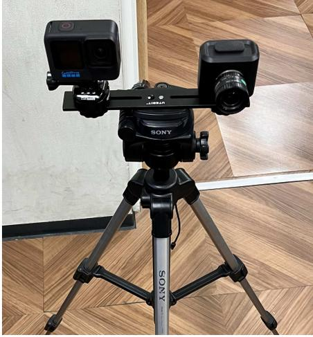
Figure 11. Device setup. On the left is the GoPro HERO 10 and on the right is Prophesee’s Evaluation Kit.
