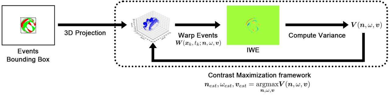
Figure 4. Overview of the proposed method. The proposed method uses the event and ball bounding box as input and normalized spin axis vector, angular velocity, and translational velocity as output. The proposed method first projects the events into a three-dimensional space by calculating the depth. Next, the parameters are estimated by iterative optimization using the Contrast Maximization framework.
