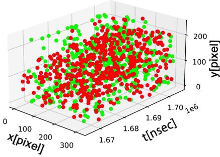
Figure 2. Example of events. The color of the dots corresponds to the polarity of the event. Events are spatio-temporally sparse point cloud-like data.
