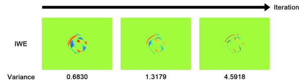
Figure 5. The process of IWE optimization. As the optimization progresses, the warp location of the event is concentrated on the edge of the ball, and the value of variance increases.
