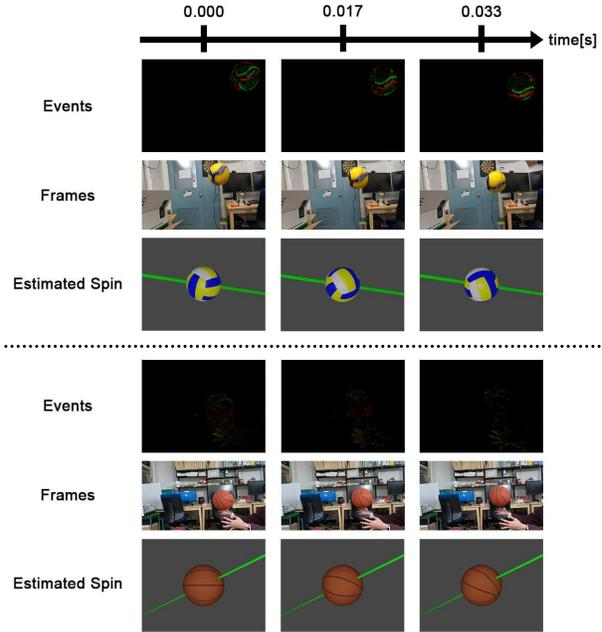
Figure 12. Qualitative evaluation on Lab Dataset. Estimated Spin images are rendered based on the estimated spin axis and angular velocity. The green line represents the spin axis.
