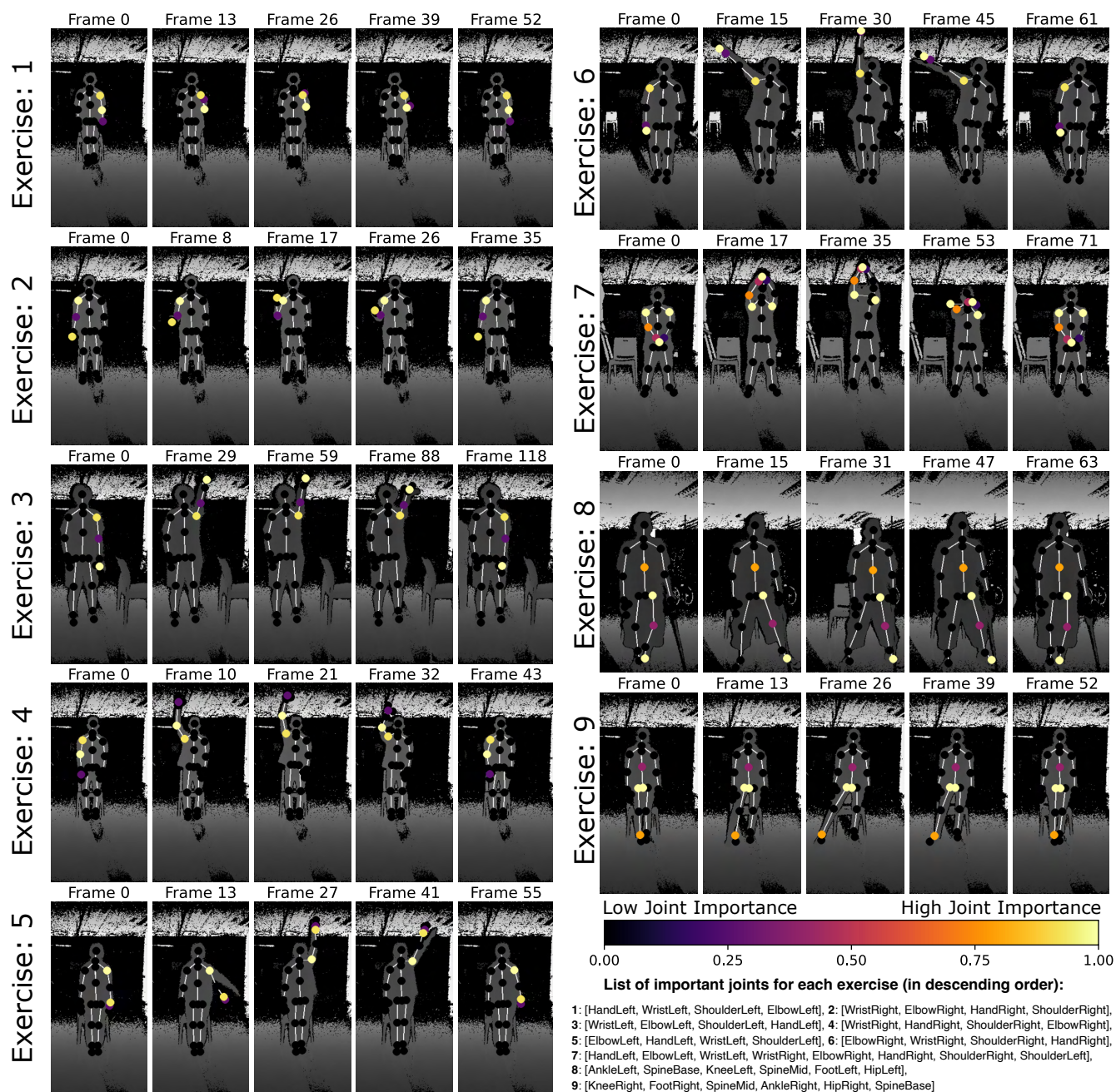
Figure 4. Qualitative analysis across a temporal sequence of frames for each exercises in standing position, with keypoints superimposed on each frame to capture the full range of motion. The heatmap gradient indicates joint importance based on RFC findings, ranging from low (yellow) to high (black), aiding in the visual comparison of execution quality. The bottom-right corner lists the most significant joints in descending order of importance for each exercise, providing a comprehensive understanding of movement dynamics.
