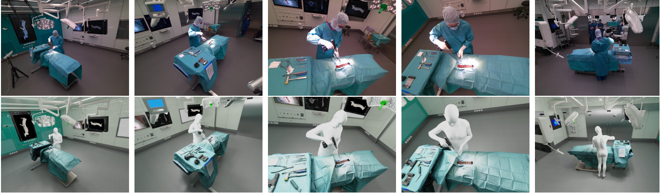
Figure 4. Comparison of the rendered digital twin with the real camera images. The camera perspectives shown from left to right correspond to the Kinect cameras 1-5 as shown in Figure 3. The digital twin was rendered in Blender using the Cycles engine.
