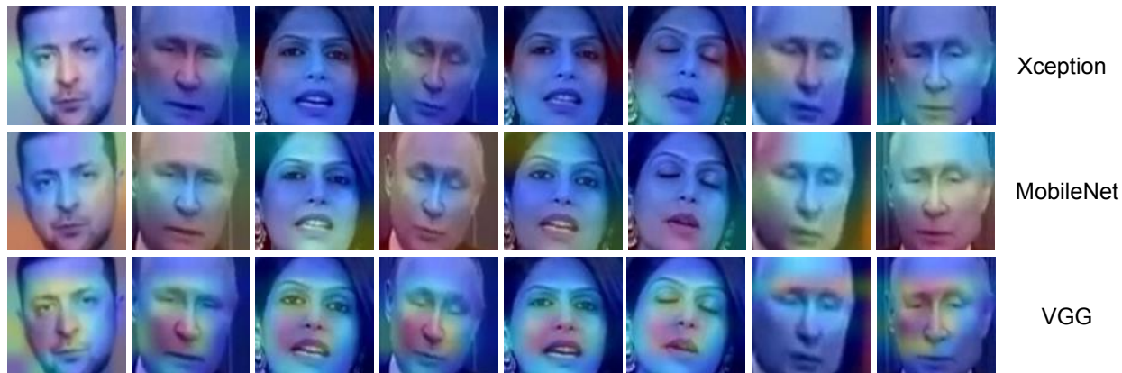
Figure 7. Grad-CAM [46] heatmap visualization reported on unconstrained images collected as part of our evaluation dataset. The heatmap information is computed using the three CNN architectures used for the development of a deepfake detection algorithm.
