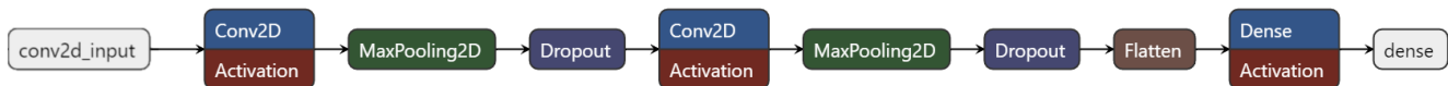
Figure 5. CNN architecture adopted for the experiments. Two 2D convolutional layers, followed by as many max-pooling layers, precede the dense layer and the two final neurons used for classification.
