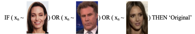
Figure 6. Linguistic rule-based representation of the prototypes for PUDD Interpretability on ‘Original’ class of Celeb-DF with top 3 closest prototypes on the feature space.
