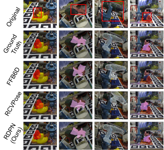
Figure 4. Qualitative results on Occlusion LineMOD. The images are rendered by projecting the 3D object model onto the image plane using the estimated pose. Our two-step dense correspondence method can accurately capture the object and predict its pose, even under heavy occlusion. This contrasts previous keypoint-based methods, which often struggle in such scenarios.
