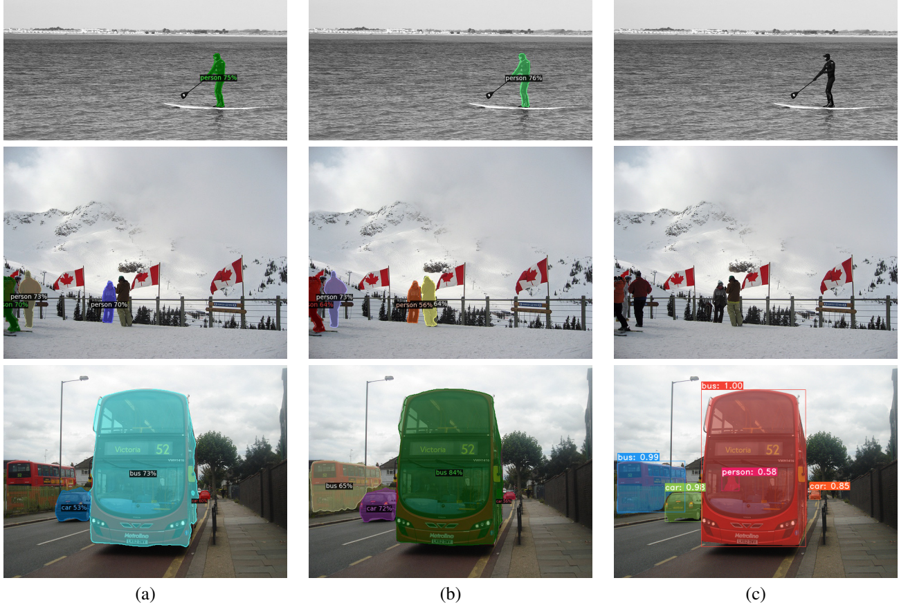
Figure 5. Some examples of instance segmentation results of (a) ConvNeXtV2-SparseInst BNN, (b) MSCAN-SparseInst BNN, and (c) YOLACT (ResNet50) [3].
