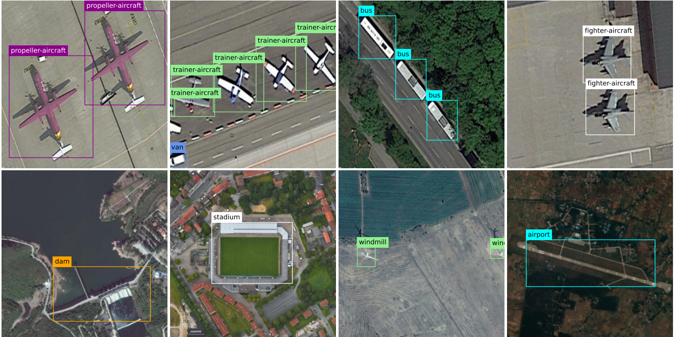
Figure 4. Illustrative qualitative results obtained by the proposed detector. Images on the top row correspond to the SIMD dataset, while images on the bottom belong to the DIOR dataset.
