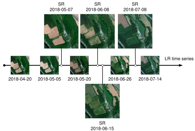
Figure 4. Multi-image super-resolution at different time steps using HighRes-net L-TAE. SR images follow changes in the LR series.
