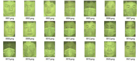
Figure 6: The PNG images are a condensed version of the MAT data, created by applying a linear transformation to reduce the image channels from 30 down to 3. This conversion is designed solely to facilitate easier visualization.
