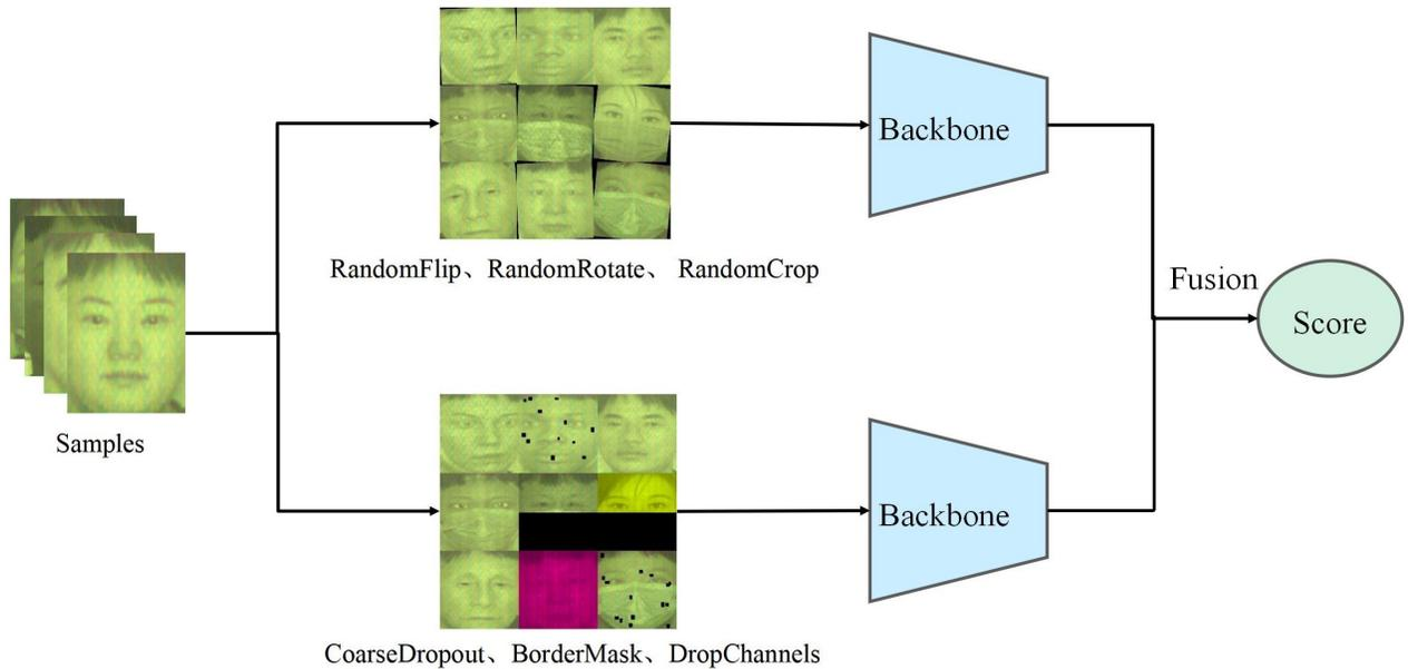
Figure 2. The framework of the proposed method. Each SSI image undergoes two different sets of augmentations and is trained by two branch models, and the outputs are finally integrated for classification.
