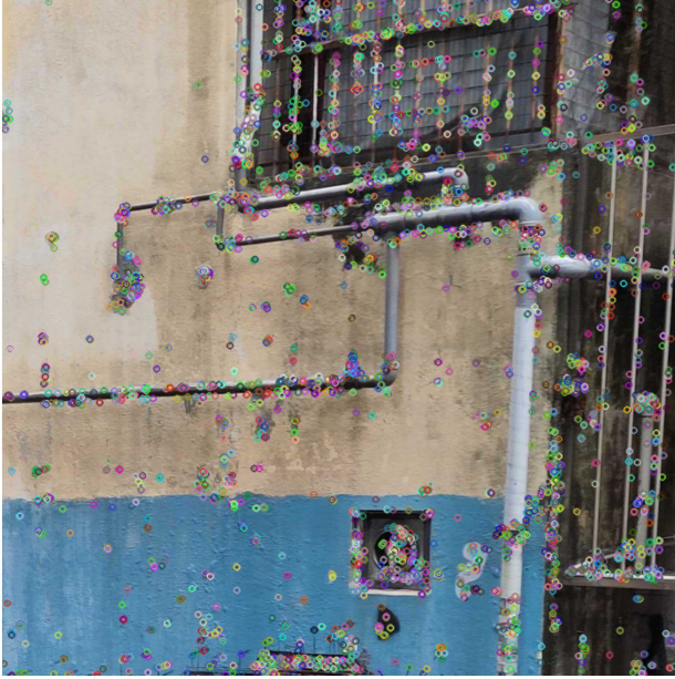
Figure 2. Clusters in DeDoDe Detections. The DeDoDe detection objective does not explicitly enforce sparsity in the detections. This has the side-effect of the network producing so-called clusters of detections in particularly salient areas of the image. This is problematic in downstream tasks, as it means that many keypoints must be sampled to ensure repeatability.
