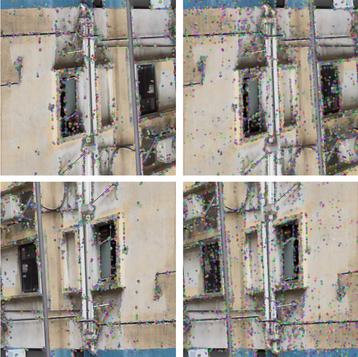
Figure 4. Sensitivity to large rotations. The original DeDoDe detector (left) is sensitive to large in-plane rotations. This was first noted by Bökman et al. [7]. We extend their ideas and additionally include joint horizontal flips. DeDoDe v2 produces more consistent keypoints under rotation of the input image (right). We plot the top 5,000 keypoints in all images.
