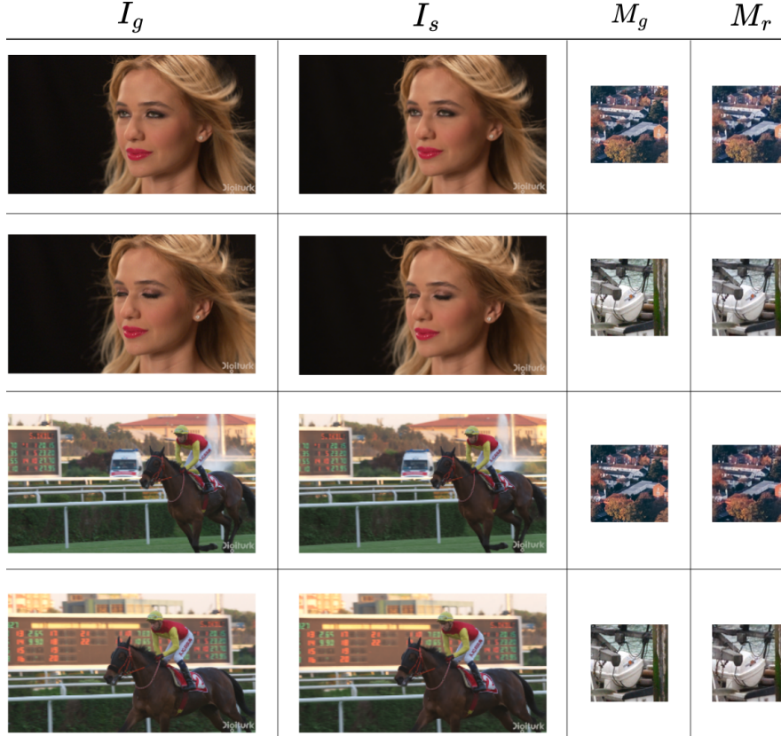
Figure 5. Subjective results for two cover videos without using attention. The two columns on the left represent the cover ( I_g ) and steganographic ( I_s ) frames with dimensions 1920 x 1080. M_g and M_r denote the ground truth and recovered hidden images respectively of size 128 x 128.
