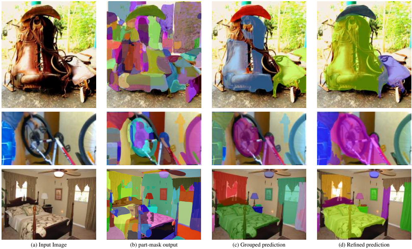
Fig. 2. Visualizing outputs after each stage of UDOS for cross-dataset training. The images in the three rows belong to OpenImages [1], UVO [2] and ADE20K [3] datasets respectively. All outputs are generated by model trained on complete COCO dataset. ((a)) shows the input image, followed by ((b)) Part-mask prediction, ((c)) grouped outputs using our affinity based grouping and ((d)) refined prediction. The masks in last two columns correspond to true-positives with respect to the ground truth.
