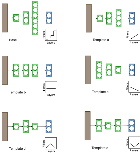
Figure 2. Schematic distribution of filters per layer in templates. Base distribution is the original pyramidal distribution. Templates follow a smoother transition in the number of filters between layers. Number of filters does not match between models but they are adjusted to fit the original number of FLOPS of the base model.
