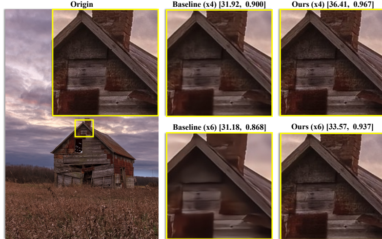
Figure 2. Illustration of RGB image compression with (baseline) and without (ours) entropy encoding loss and auto-regressive module for side information. Evaluation metrics are shown as [PSNR, SSIM]. For both compression at 4 and 6, training RGB image compression without entropy encoding yields better image quality with finer details.
