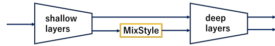
Figure 2. Internal Structure of the Feature Extractor. MixStyle is applied to random shallow layers of the CNN, and domain information is mixed across batches.
