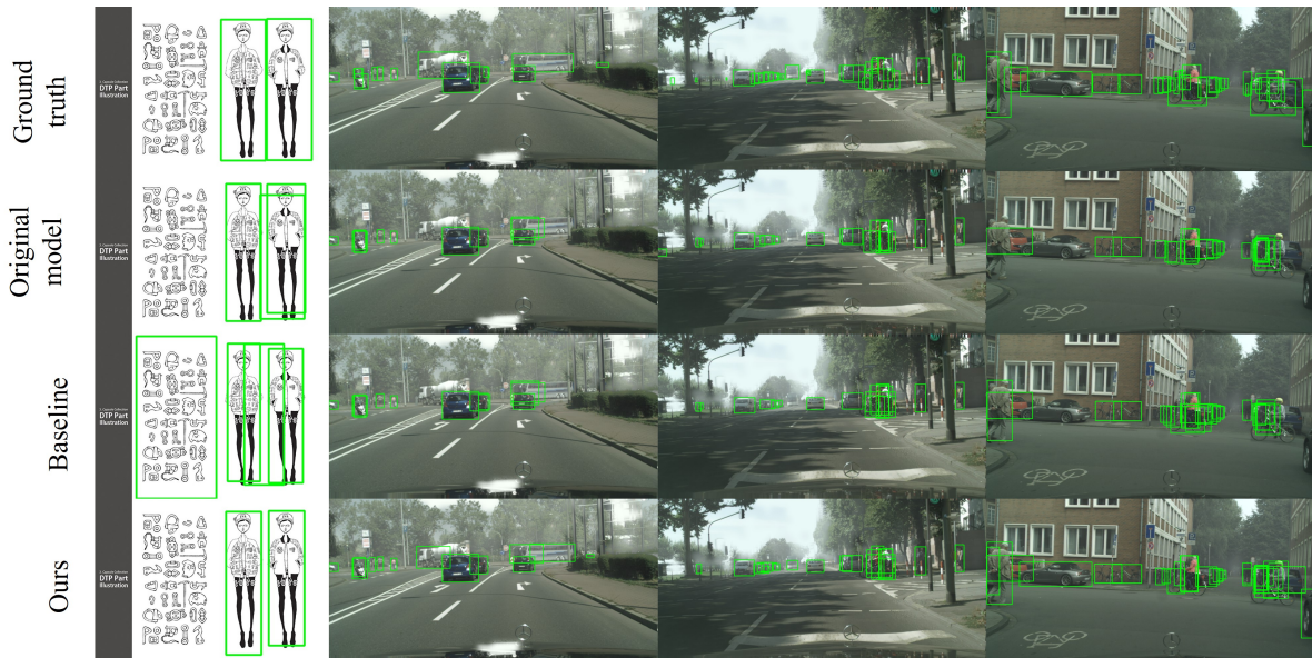
Figure 1. Qualitative results of fully test-time adaptation for object detection. The first row is the ground truth of each image, the second row is the results of the pre-trained detector, the third row is the results of the self-training baseline, and the last row is the results of our proposed method. All the object detections are denoted as green boxes.
