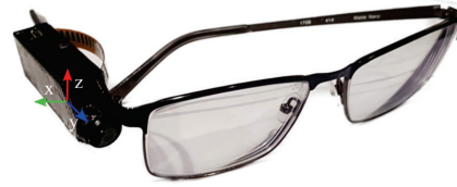
Figure 2. AIM-2, an egocentric wearable camera that monitors ingestion behavior.
