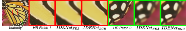
Figure 6. Visual comparison of Wiener Filtering in feature and RGB space on Image 'butterfly' ( \times 4 ) from Set5 dataset. The kernel width is 3.2.
