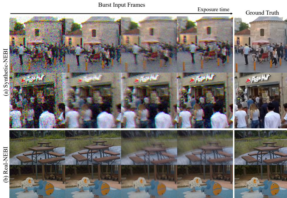
Figure 3. Visualization of the Synthetic-/Real-NEBI dataset. The left four columns display a subset of 14 input bursts, while the rightmost column presents the ground-truth image corresponding to the first input frame. From left to right in the burst sequence, the exposure time increases, resulting in decreased noise and increased blur. Best view to zoom.
