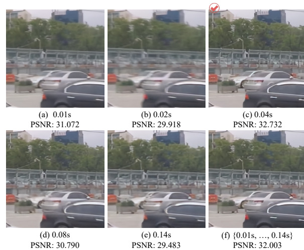
Figure 1. Output quality decreases when a BISR model uses burst shots taken at sub-optimal exposure times compared to optimal time (c). On the other hand, as shown in (f), the model reconstructs a high-resolution (HR) image as if it were captured using optimally exposed burst shots by harnessing information from non-uniformly exposed burst shots.
