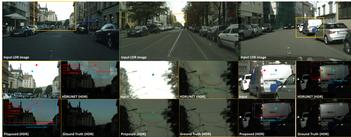
Figure 1. HDR reconstruction from a single LDR image. By learning the receptive field of each overexposed pixel location so that the receptive field can include non-overexposed information for restoring a overexposed object properly, our method restores the overexposed objects such as power lines, a car and sky accurately. These differences are better visible in pdf version with zoom-in.
