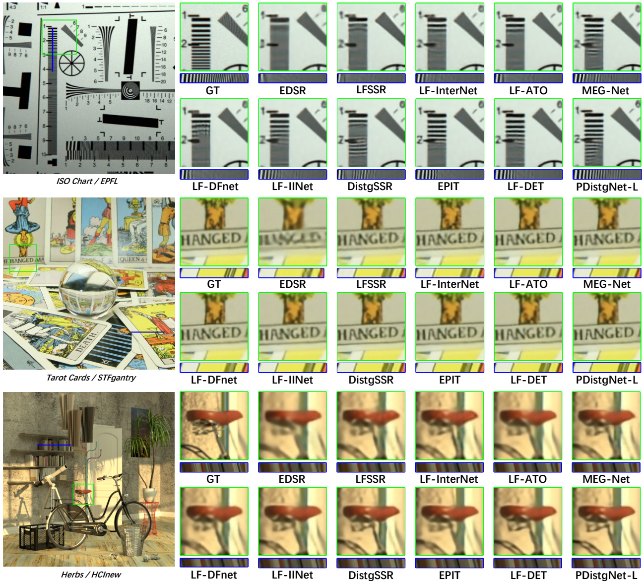
Figure 4. Visual Comparison on different methods for 4\times LF image SR. The enlarged patches cut from the green box of central view and epipolar-plane image cut along the blue line are presented for comparison.
