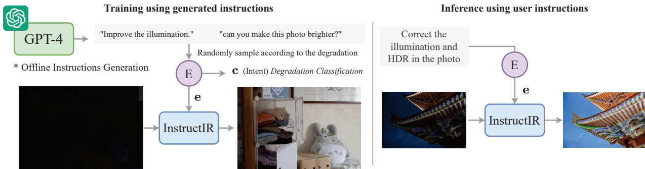
Figure 13. InstructIR [23] takes as input an image and a human-written instruction for how to improve that image. The multi-task model performs text-guided low-light image enhancement.
