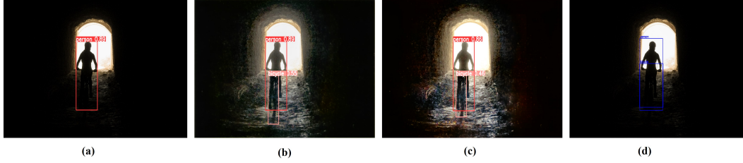
Figure 5. Accelerating OD performance on edge devices by leveraging proposed optimization framework. (a) Low-light image with YOLOv3 [34]. (b) Our model (INT8) with YOLOv3 [34]. (c) Our model (full precision) with YOLOv3 [34]. (d) Ground-truth (for detection)
