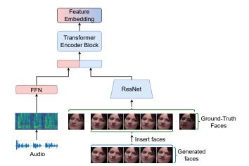
Figure 3. In the training, since extracting features from entire videos provides more informative features [41], we insert the generated faces into the corresponding part in the target video. Then, we use this video for feature extraction after cropping the mouth.
