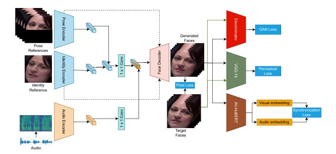
Figure 2. Illustration of the proposed audio-driven talking face generation model and employed loss functions.
