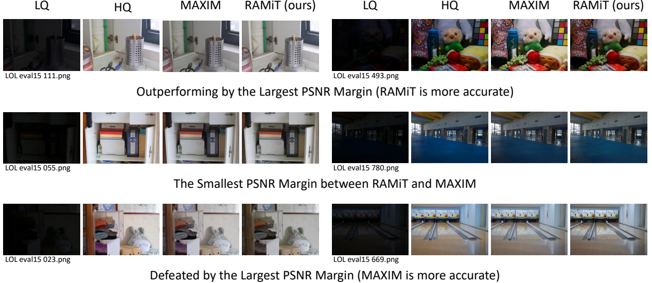
Figure G. Visual comparisons of MAXIM [33] and RAMiT. Despite even fewer parameters, RAMiT can restore the extremely dark images with better or matched accuracy compared to MAXIM. In the bottom row, the cases in which RAMiT is highly defeated by MAXIM are provided as well.
