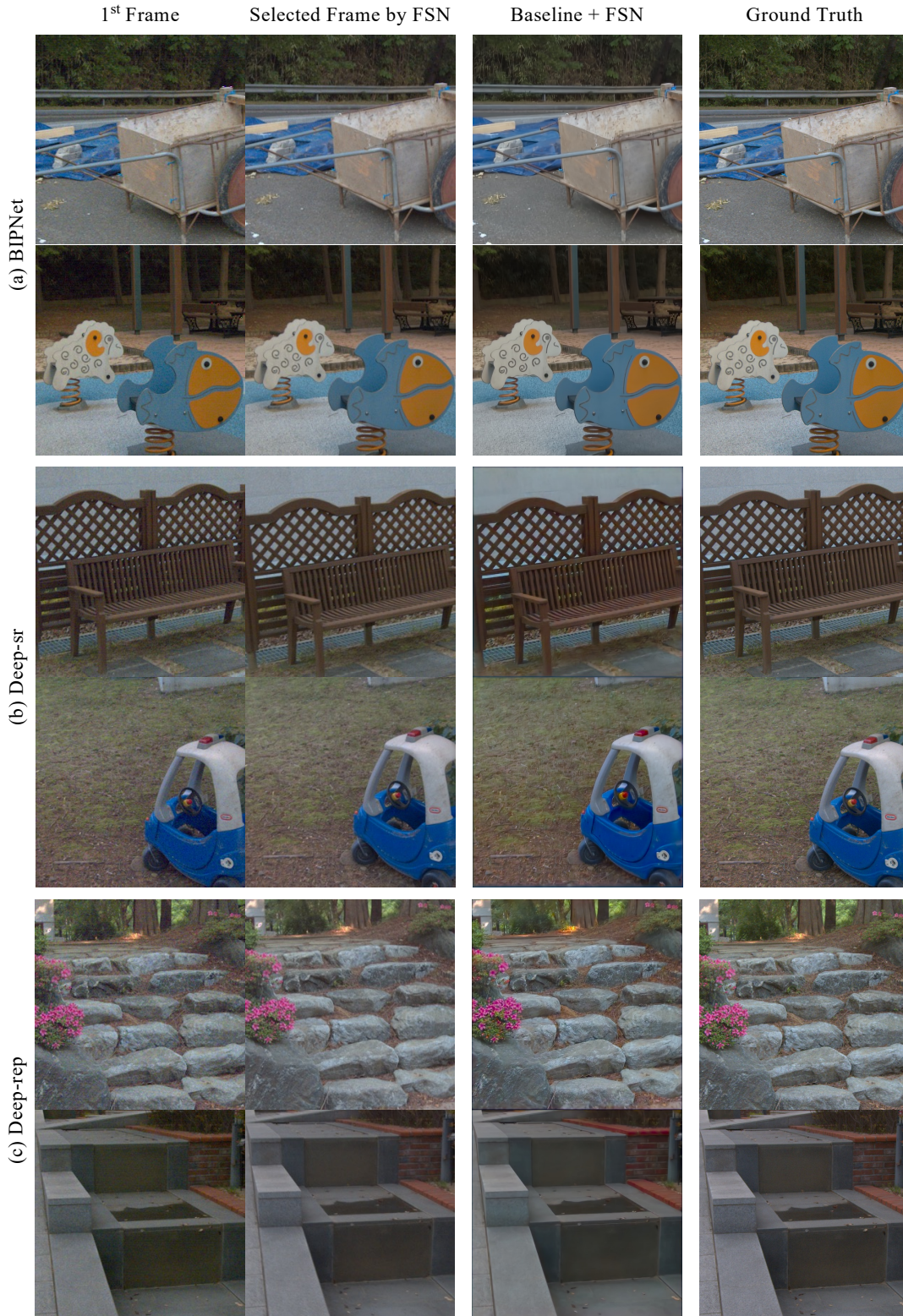
Figure 7. Qualitative comparison on synthetic-NEBI. We present the results of three previous methods—(a) BIPNet [4], (b) Deep-sr [1], and (c) Deep-rep [2]—with the FSN. 'Baseline + FSN' indicates the integration of the FSN on top of the baseline in a plug-and-play manner. The FSN selects a frame with less noise than the 1 st frame well, resulting in improved visual quality. Best viewed when zoomed in.
