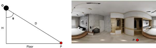
Figure 5. For any point  $P$  on the floor, the distance  $D$  from camera  $O$  to  $P$  can be calculated from the camera height  $H$  and angle  $\theta$ , composed of planes. The segmentation pipeline and results are shown in Fig. 4, where different colors on the walls represent different masks classified as wall segments.
