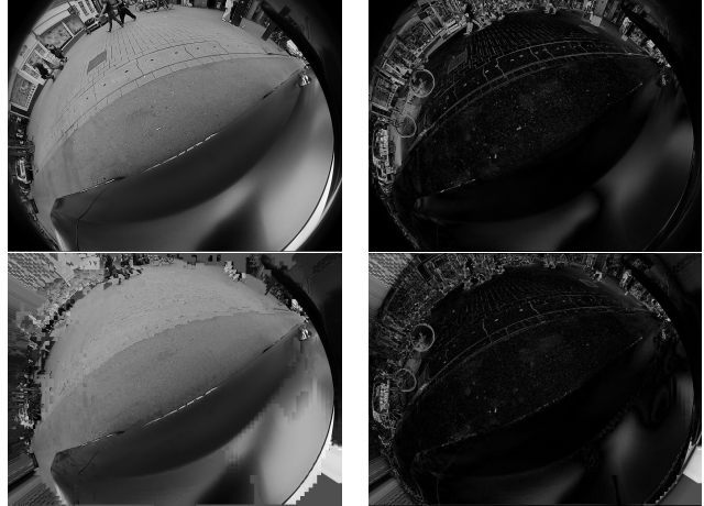
Figure 10. WoodScape MVR: Full prediction gray images and errors images corresponding to zero motion predictor and epipole guided locally affine predictor. Top row zero motion predictor with error image (MSE 1372). Second row, epipole guided 16x16 locally affine predictor and error image (MSE 1269).
