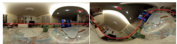
(e) Equirectangular images: (left) image obtained with the camera at an upright posture; (right) image obtained at the same position with an inclined camera.
