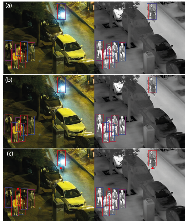
Figure 7. Visible and IR image pair from the LLVIP test-set. (a) is CAFF detection, (b) is concatenation, (c) is cosine-similarity. Ground-Truth are framed in red while our model's detection are framed in blue. Confidence threshold is 50 %. A red triangle indicates the missed detection.
