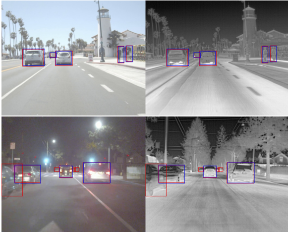
Figure 5. Visible and IR image pairs from the FLIR-aligned test-set. Ground-Truth are framed in red while CAFF-DINO detection are framed in blue (confidence threshold set to 50 %).
