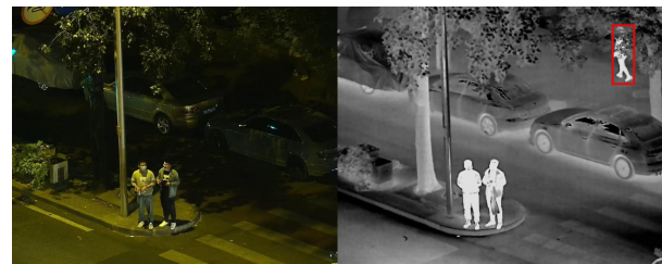
Figure 1. From left to right: visible and IR image patches from LLVIP dataset in low-light situation [5]. The reduced enlightenment illustrates the benefit of IR: the third pedestrian, framed in red, is barely noticeable in the visible spectra.
