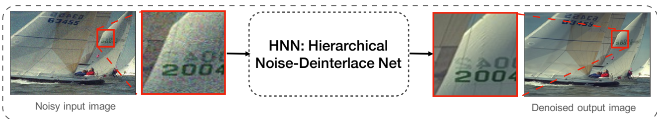
Figure 1. Framework of Hierarchical Noise-Deinterlace Net (HNN) for image denoising. The zoomed-in view (red color) shows specific area of exemplar image.
