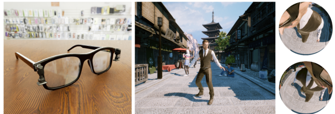
(a) Dataset setup for UnrealEgo [3]: Left image shows a glass equipped with two fisheye cameras. The middle image provides a third-person perspective of the person, offering context to the scene. The right image depicts the egocentric view of the person.
